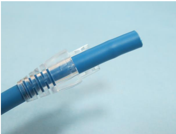
3. Insert BOOT into the cable .
