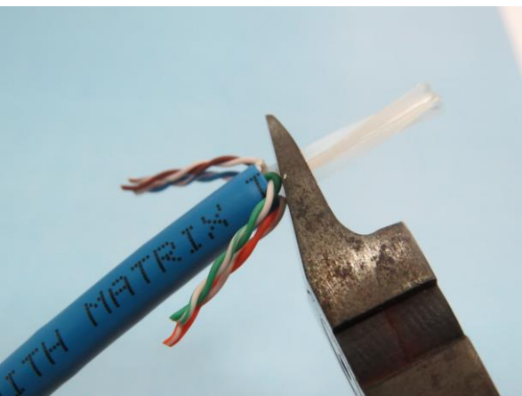
5. Trim cable cross member and separate four pairs.
