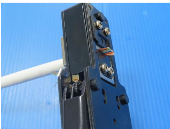
9. Put the assembly into feed through tool PM-3008R
