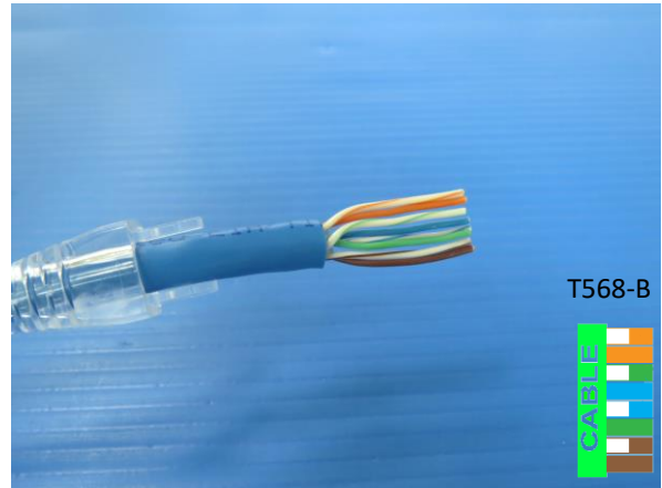
5. Untwist the wires. Arrange the wires according to TIA/EIA 568A & 568B standards.
