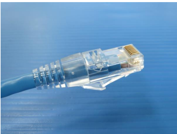
9. Push the boot SR-032M into plug.
