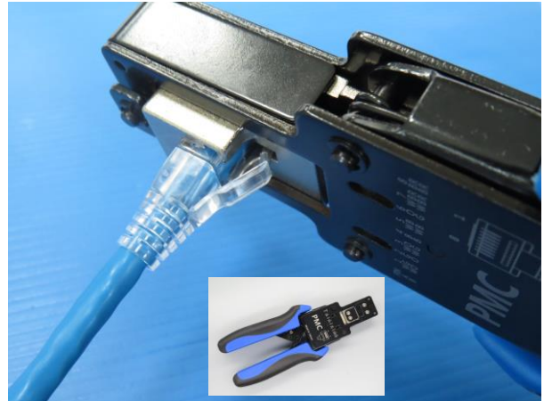
10. Insert the plug into crimp tool. Firmly squeeze the handles to set the contacts and secure the cable.
