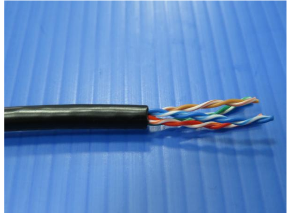
2. Strip and removed 20mm of jacket.
