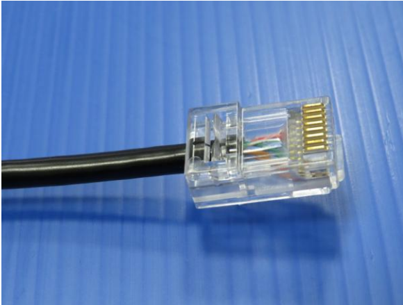
7. Slide assembly into the plug body.
