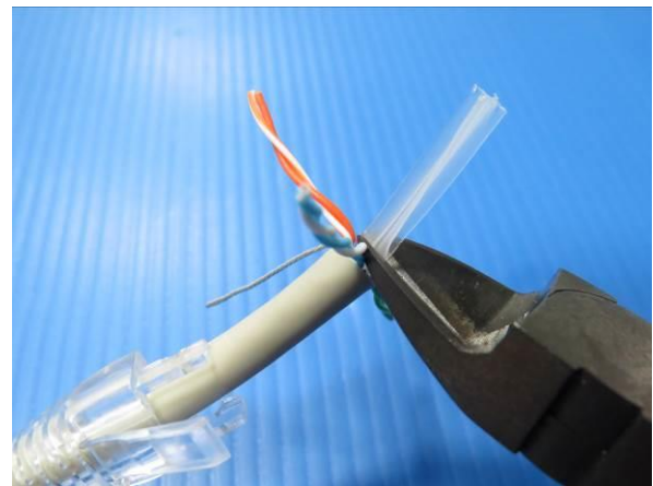
5. Cut off the tinfoil , Trim cable cross member and put drain wire down to avoid interruption.
