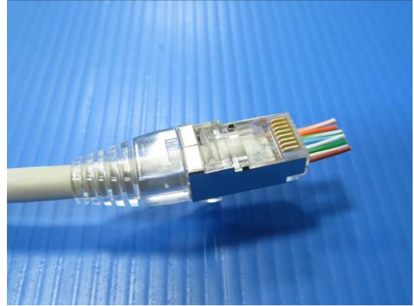
10. Push boot into plug body.
