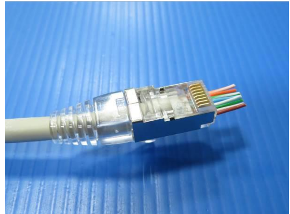
10. Push boot into plug body.
