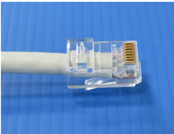
8. Slide the assembly into PLUG body. (Push inside as you can)
