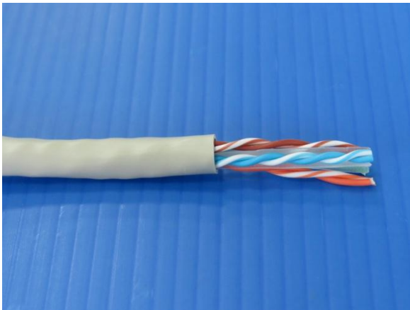
2. Strip and remove 20mm of jacket.
