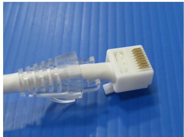
6. Slide assembly into plug body.
