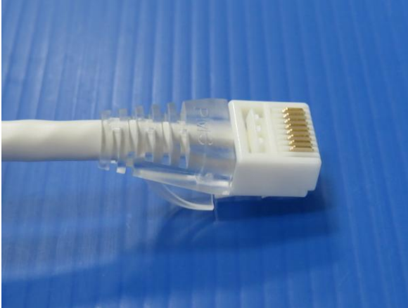
7. Slide boot into plug body.
