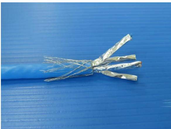
3. Put copper woven mesh down to avoid interruption .
