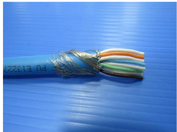
4. Cut off the tinfoil and twist drain wire for welding.
