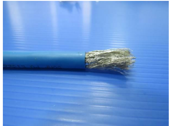
2. The Cable PVC 20mm by stripping.
