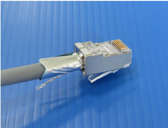
7. Slide assembly into plug body.
