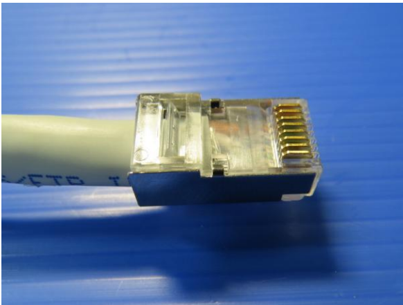
9. Push the cable and insert into PLUG body.
