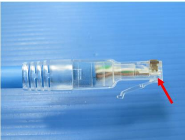
15. The wires are not pushed in place yet. ( Please note the arrow .)
