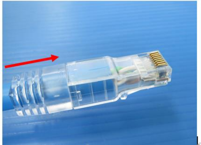
16. Push the cable again to send wires to the front.
