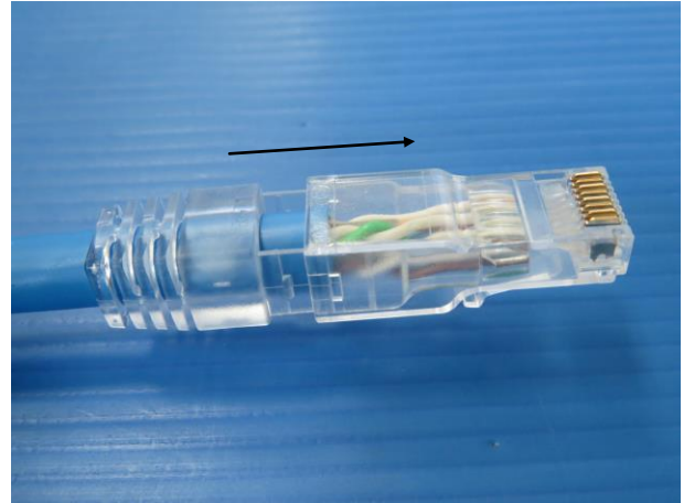
14. Push the assembled wire into the PLUG. ( Priority push the Boot into plug body to fix it )
